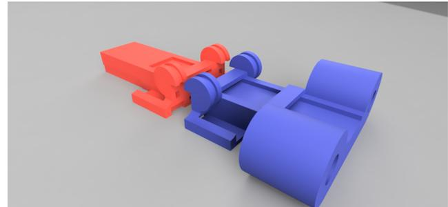
Fig. 3. Rendering of the two parts of the mechanism that sit on opposite sides of a finger joint. A piece of steel sheet metal slides through the channel in the blue piece and anchors into the corresponding channel in the red piece. The circular sections serve as pulleys to route the string. The small channel on the side holds the inverse stiffness spring.
