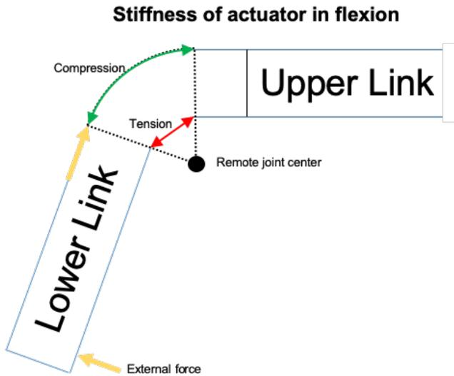
Fig. 4. Depiction of the flow of forces under an external force trying to extend the exoskeleton. The steel sheet metal (green) acts as an arch under compression, making it very rigid. The string (red) remains in tension.
