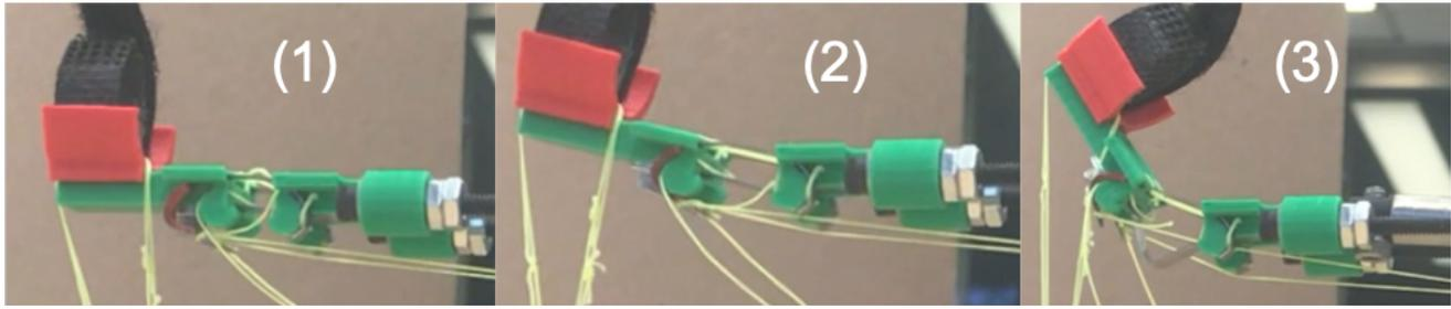
Fig. 6. The three states, corresponding to two stages, of the actuation process. In (1), the mechanism is in its most collapsed form and the string is not taut. The linear actuator pushes on the lower link (on left), which purely translates until the string becomes taut (2). Subsequent force applied by the linear actuator forces the mechanism to purely rotate (3) about a remote joint center.
