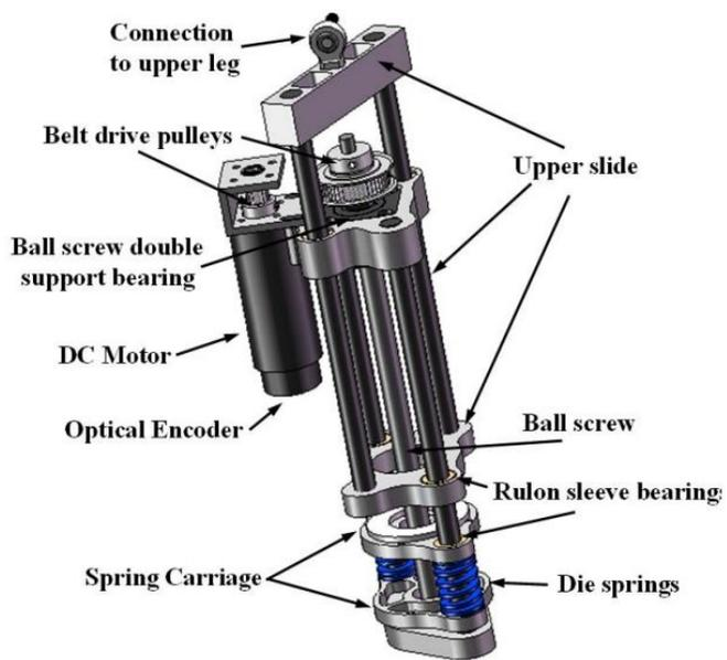
Fig. 8. CAD model of the actuator module.
