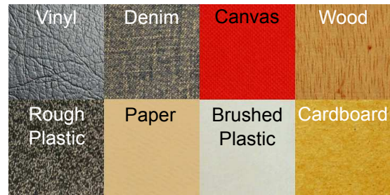
Fig. 1. The eight materials that were haptically modeled with the methods presented in this article. Each surface has unique microscopic details that induce distinctive vibrations when contacted with a probe.
