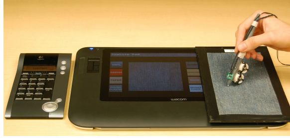
Fig. 9. The Wacom tablet (center) displaying the haptic texture user-study software, and the real texture mounted alongside it (right).
